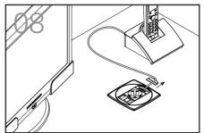
The unit system can be used to access a cable tray by simply removing a tab, diagram 8.
