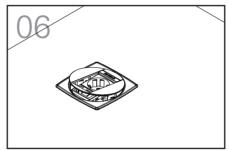
When the unit is fixed, put the cover back on, as shown in diagram 6.
