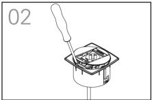
Use a fine head screwdriver to remove the cover of the anchor mechanism, as shown in diagram 2.
