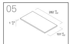
**BOX PLUS COVER LAYER**: To cover the Box Plus cover with a finish that matches the desk (wood or another material), cut a layer with the same dimensions shown in figure 5.
