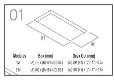
**IMPORTANT:** Do not exceed the tolerance dimensions or the product will not be installed properly.
