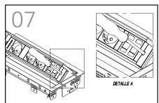
Insert a flat-head screwdriver into the holes in the rail tabs, levering, always towards the outside of the box.
